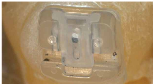
Fig. 8. Damon Clear after 300,000 cycles at ~40 N.
