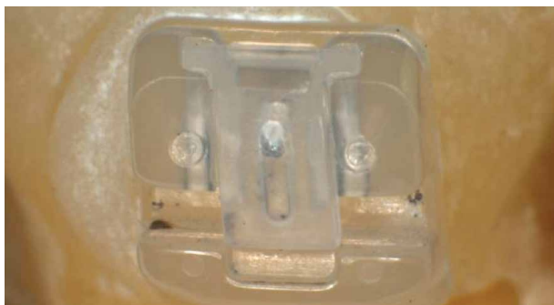
Fig. 7. Damon Clear after 200,000 cycles at ~40 N.
